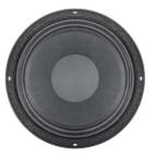
The MBX series mid-bass woofers from B&C Speakers offer acoustic designers a new range of high efficiency, wide bandwidth alternatives that are not currently available in the B&C range. These full-featured transducers incorporate lightweight neodymium motors, inside/outside wound copper clad aluminum wire voice coils, weatherproof impregnated paper cones, and a symmetrical inductance profile. The MBX Series is especially well suited for two-way loudspeaker enclosures.
