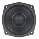
For simplified cabinet assembly and efficient thermal transfer to the air, our NSM series of sealed back midranges feature a cast aluminum sealed chassis, high strength neodymium motor, and large internal volume for good low frequency performance. Large voice coils provide power handling, while careful selection of suspension and cone components results in exceptional sensitivity. These dedicated narrow-bandwidth midranges offer the lowest distortion at given output of any midrange available.
