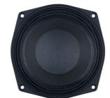
The MBX series mid-bass woofers from B&C Speakers offer acoustic designers a new range of high efficiency, wide bandwidth alternatives that are not currently available in the B&C range. These full-featured transducers incorporate lightweight neodymium motors, inside/outside wound copper clad aluminum wire voice coils, weatherproof impregnated paper cones, and a symmetrical inductance profile. The MBX Series is especially well suited for two-way loudspeaker enclosures.
