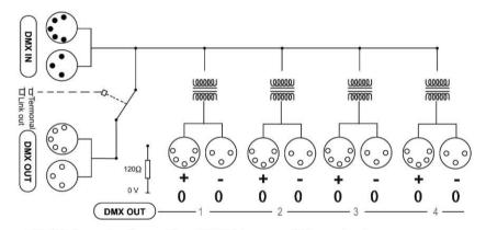
DMX input : from the DMX transmitting device DMX output : connect to the DMX receiving device
