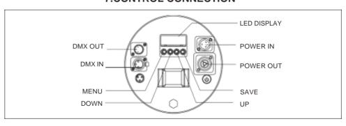
Connect the provided XLR cable to the female 3-pin XLR output of your controller and the other side to the male 3-pin XLR input of the moving head. You can chain multiple Moving head together through serial linking. The cable needed should be two core, screened cable with XLR input and output connectors. Please refer to the diagram below. DMX-512 connection with DMX terminator.
