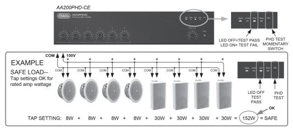
The Fault LED should never be constantly illuminated or damage may occur to the amplifier or sound system. If the Fault LED comes on steadily during use or during the PHD test there are a few common fault conditions to check if using a 100V distributed audio system.
