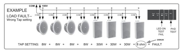
B. Check each speaker to be sure the load tap is set to the correct power setting. The total power tap selected of all the speakers combined should not exceed the amplifier's maximum power rating or a fault may occur.
