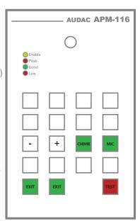
The volume for the Microphone can be adjusted by pressing the "Mic" button and pressing the "+" and "-" buttons for increasing or decreasing the volume. To test if the delected volume is correct, you can press the orange "Test" button, whereafter the voice speaking into the microphone will be heard.
