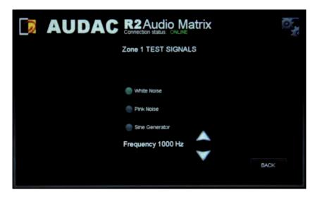
When one of the test signals is selected, "Other" will appear in the 'Input Selection" box on the main screen.
