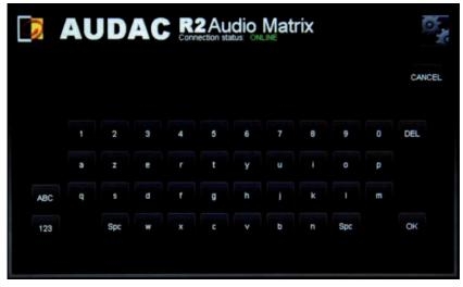
A password should be entered to get access to the R2 amplifier. There are two different access levels, administrator level and user level.
