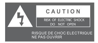
The lightning flash with arrowhead symbol within an equilateral triangle, is intended to alert the user to the presence of uninsulated "Dangerous Voltage" within the product's enclosure that may be of sufficient magnitude to constitute a risk of electric shock to persons.
