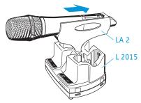
▶ Plug the LA 2 charging adapter with the inserted radio microphone into the L 2015 charger (see "Accessories and spare parts" on page 30).
